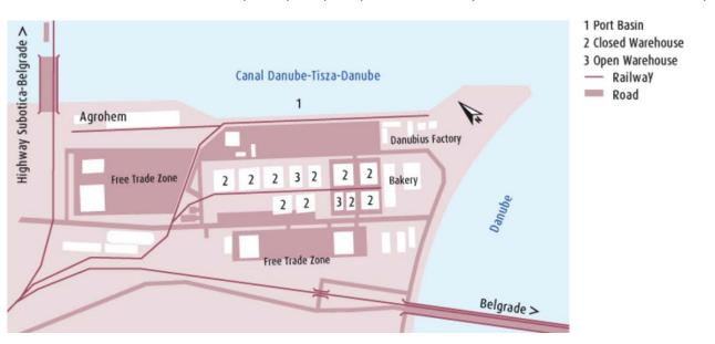
The port has 5 deep-water berths, with the possibility of mooring 5 ships at the same time. The mooring front is 1600 meters, where the mooring front is 800 meters, and the sloping coast is 800 meters. The maximum depth at the berth is 3.0 meters. There are reloading facilities: portal cranes - 4/5 - 27.5. Warehouse area: covered - 40,000 sq.m., open - 100,000 sq.m. There is also a rail connection.
