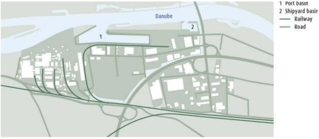
The port of Kelheim-Saal consists of a 675 m long quay parallel to the Danube in an east-west direction and a 120 m turn basin in the inlet area. Transport-intensive companies settled along the transshipment banks.
