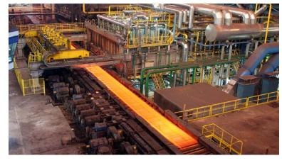
refining in a 100-tonne ladle furnace and a vacuum degasser. Cast iron, scrap, and alloying additives are used to smelt many types of stainless steel, which are raw materials for the production of end products.
