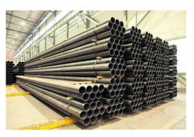
323.9 mm, with wall thicknesses from 3.0 mm to 12.7 mm and unit lengths from 6 m to 18.0 m, as per PN-EN ISO 3183, PN-EN 10217-1/2, PN-EN 10224 and PN-EN 10219-1/2 standards both in Poland and abroad.,
