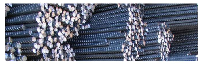
The mill is a rolling line with a nominal capacity of 360,000 tonnes, with a continuous arrangement suitable for the production of concrete reinforcement and round bars in the size range of 8-40 mm, as well as for the production of wire rods in the 7-14 mm range.
